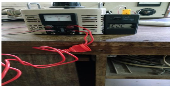
Figure 6: Experimental Set-Up (Voltage Regulator and Digital k-type Thermocouple)
