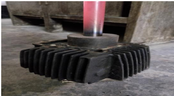
Figure 5: Experimental Set-Up (Engine Cylinder and Cartridge Heater)
